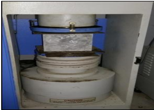
Fig. 4: Test setup for compressive strength test
