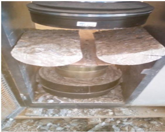
Fig. 9: Test arrangement for tensile strength
