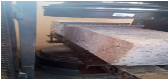
Fig. 14: Flexural test arrangement
